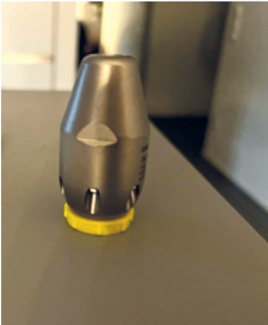
Flushing nozzle (ENZ company)
